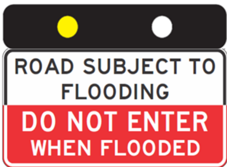
Figure 9(b) – Roadway flood monitoring system signage showing advanced warning flooding warning lights – TC1768 and TC2316
