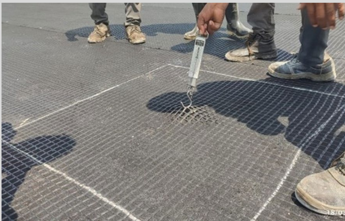
Figure 10.2.4 – Spring balance test to measure the construction bond strength
