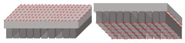
If unable to measure the underside of the girders / deck units, calculate the pre-camber values from the differences between the set out height deck surface and As Constructed deck surface height
