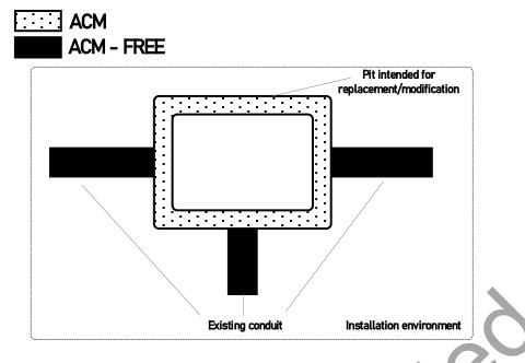
Figure 6.1.1(b) – Scenario 2: ACM pits in contact with ACM-free conduits
