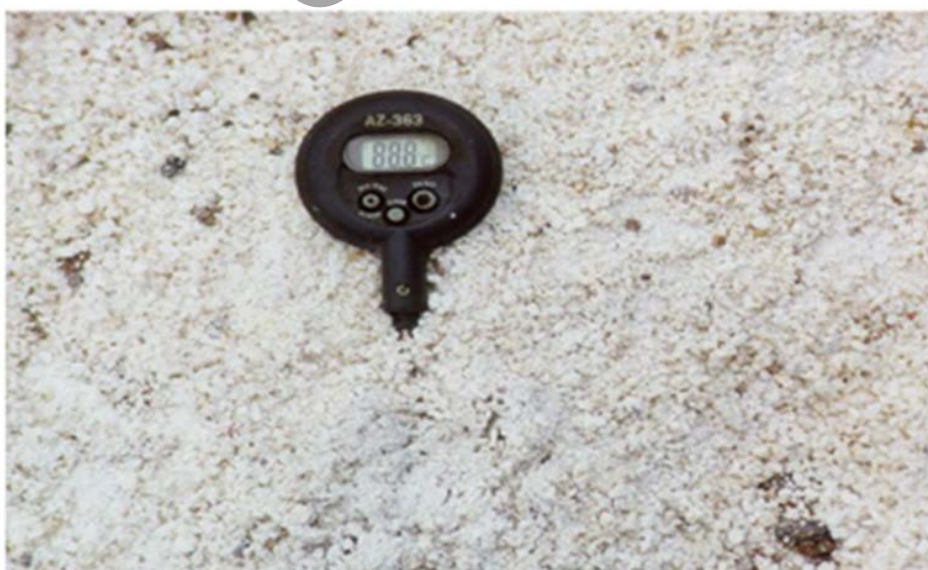
Figure 8.7.5.3 – Checking completion of slaking with temperature probe
