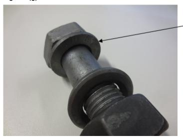
The writing on the washer is placed against the steel work.
