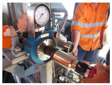
Figure 8.2(b) - View of the nut end in the skidmore
