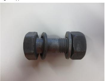
Figure 5(g) – Washers are installed so the chamfered face is against the turning surface
