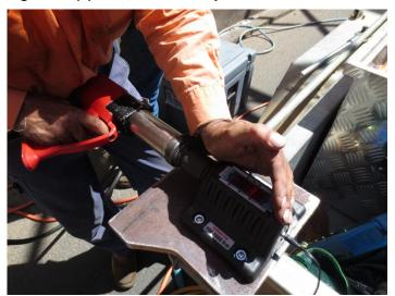
True Checker device is used to outline the torque setting for a torque wrench. Many wenches are set via pressure and the true checker determines the torque in the torque wrench for a specific pressure. True Checker can also be used to ensure the torque in the torque wrench correctly calibrated.
