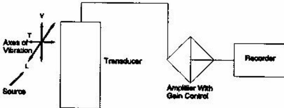
The Vibration Measurement system consists of three basic components:
