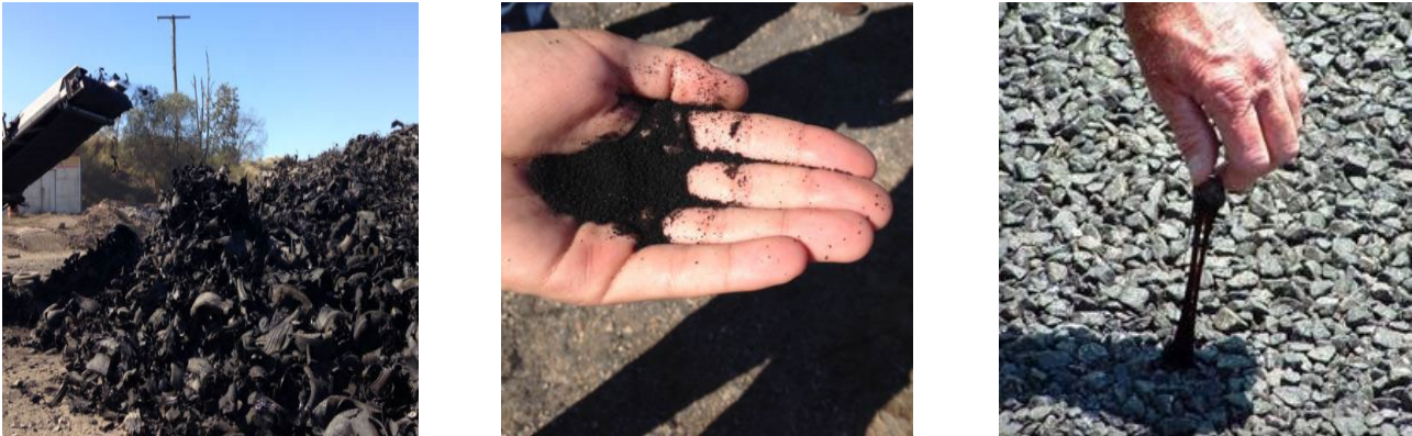
Figure 2.1 – From tyres to crumb rubber to CRMB
