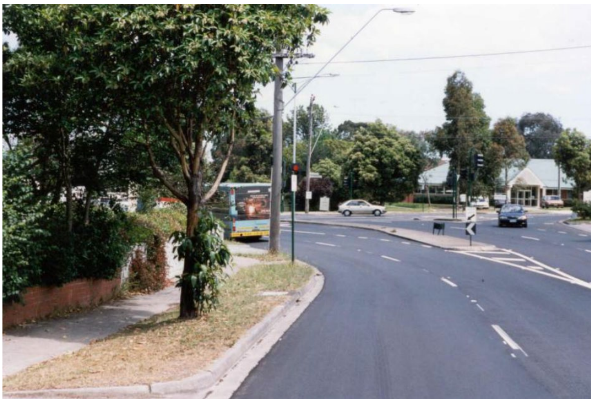
Figure D.6 – Vegetation obstructing signal on the southbound approach curve
