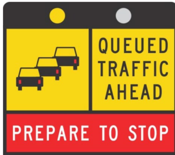
Figure 2.2(c) – Static queued traffic ahead sign supplemented with alternating wig-wag lights
