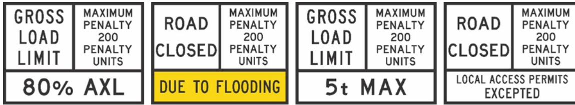
Figure 4.2.2(b) – Examples of multi-message signs in accordance with the Transport Infrastructure Act 1994.
