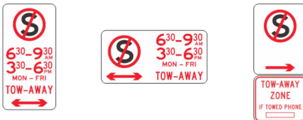
Alternatively, where it is desired to provide drivers of towed vehicles with contact information for recovery of their vehicles, the TOW AWAY ZONE sign (R5-Q01) may be used in lieu. This sign is mounted immediately below the relevant linear parking control sign as shown in Figure 3.3.2.
