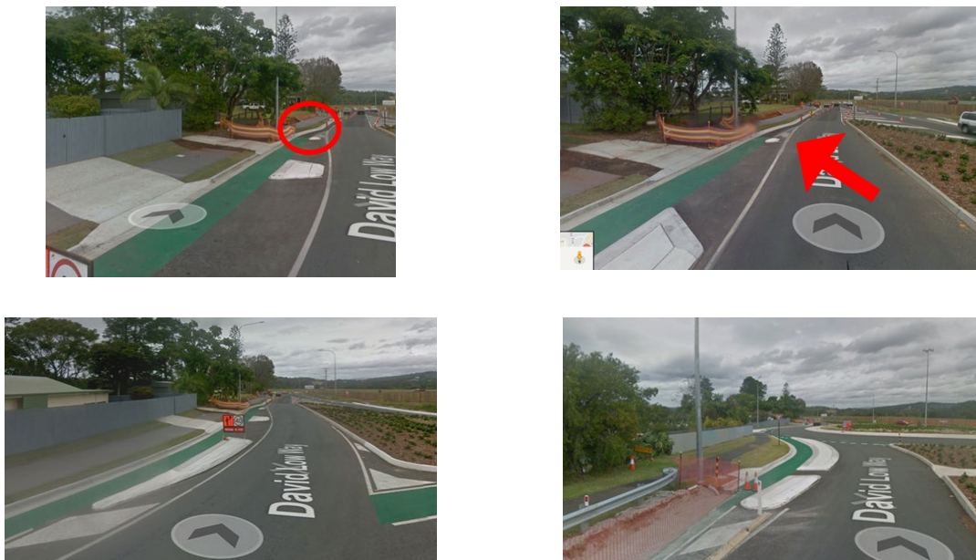
Figure 4.1.1 – David Low Way: Showing concrete islands separating the bicycle lane from the road
