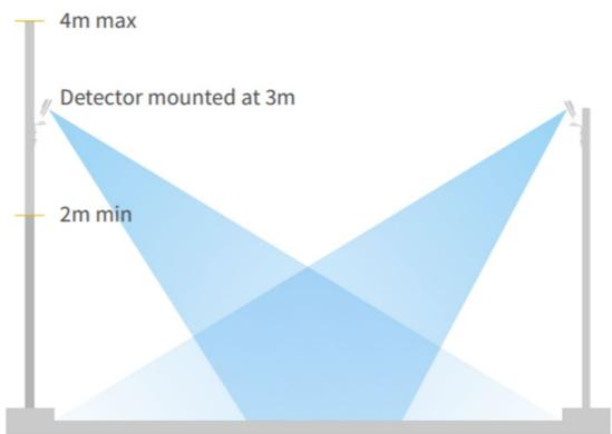
Two detectors per carriageway are required as the detector does not cover the area directly under the post it is mounted on. Transport and Main Roads uses the two detectors to detect misalignment of the radars that might not otherwise be detected as a fault.
