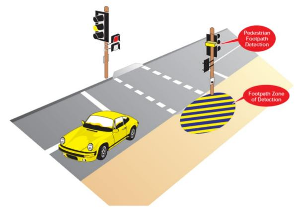
Detailed information should be sought from suppliers regarding the detection range and mounting height. Incorrect height or mounting may cause malfunction of detectors and risk to pedestrians.
