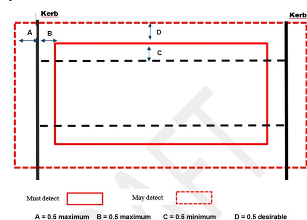
Figure 5.3 – Minimum zone of detection
