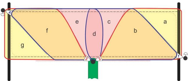
Figure 5.2 – Typical detector coverage of a divided crossing
