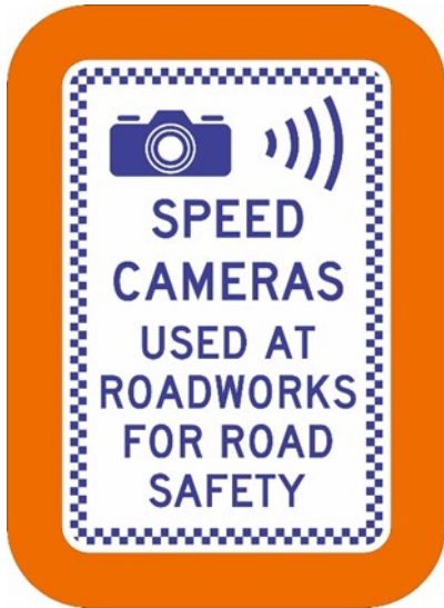
Figure 5.5.4(c) – Traffic Control sign TC2320_1 for speed enforcement planned and undertaken in accordance with Technical Specification MRTS02 Provision for Traffic
