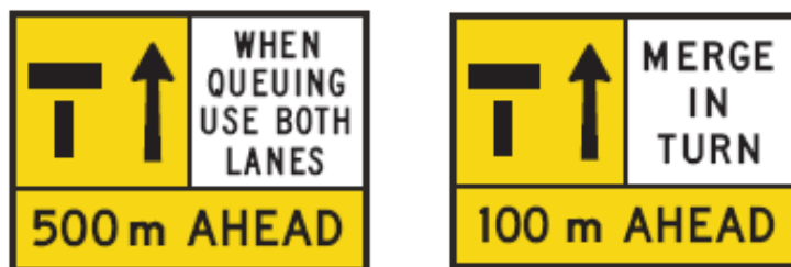
Figure 4.8(c) – Multi message sign assembly examples for multiple lane queueing (sign located on left side of the road)
