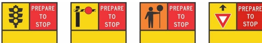
Figure 4.8(b) – Multi message sign assembly examples (sign located on left side of the road)
