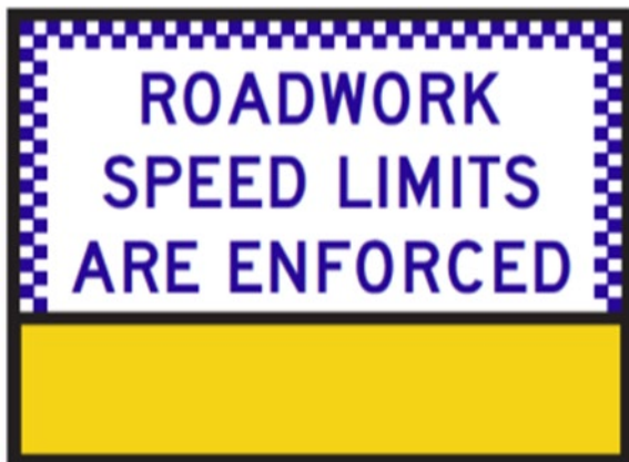
Figure 5.5.4(b) – Multi-message sign arrangement for planned enforcement by other than a camera (undertaken outside the requirements of Technical Specification MRTS02 Provision for Traffic)
