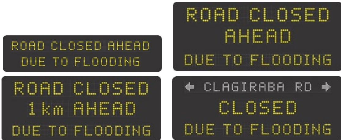
Figure A.5.2 – Example electronic sign arrangements for advance warning of a road closure
