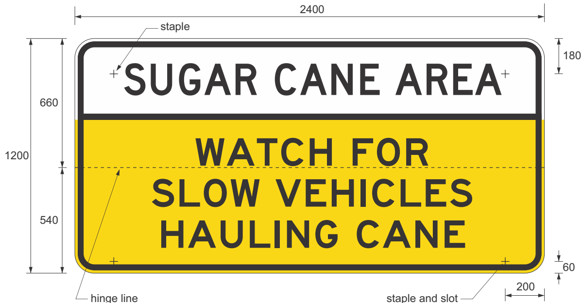
G9-Q03_3A (Option A) HINGED FLAP IN LOWERED POSITION
