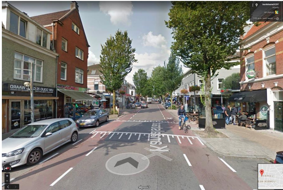
Figure 3.1(c) – Advisory Bicycle Lanes – Example from Kanaalstraat, Utrecht, Netherlands (Source: Google Streetview)
