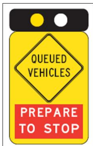
Figure 4.5.3 – Advance queue warning sign
