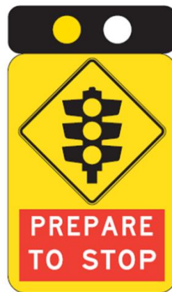
Figure 4.5.1 – Ramp signal warning sign with flashing lights
