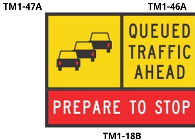
Figure 4.8(a) – Queued traffic ahead multi-message sign assembly
