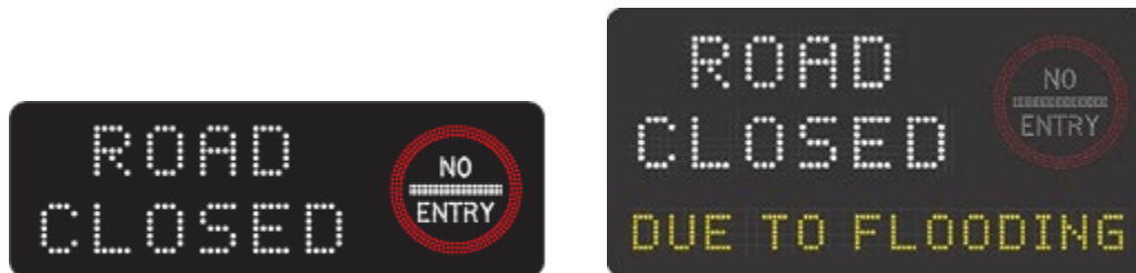
Figure A.3.2 – Example electronic VMS sign arrangements for closing a road
