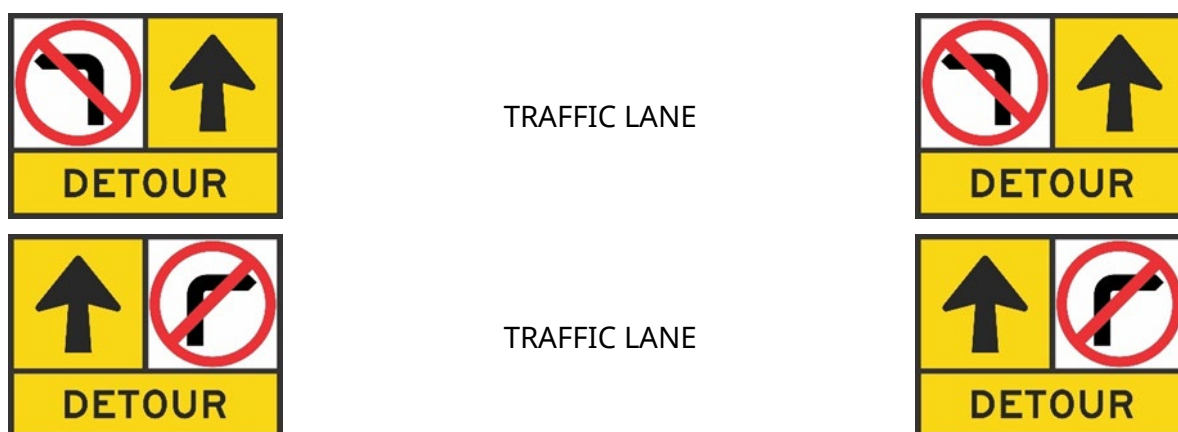
Figure 4.2.2(a) – Example multi-message signs with No Left / No Right Turn prohibition panels
