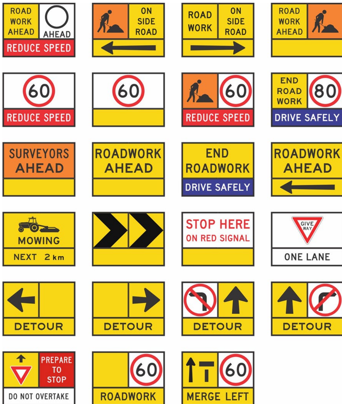
Figure B2 – Additional multi-message sign combination examples with traffic travelling to the right side of the signs
