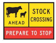
Please note – the external borders will be a folded metal frame of the type normally used for a temporary sign. Only the internal borders will be marked.
