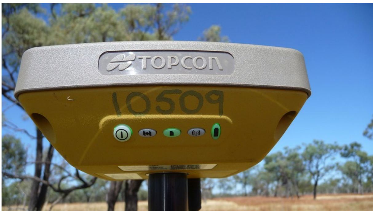
Photo 2b – The shortened serial number usually used in the file name (marker pen on side of receiver/antenna). This helps correlate the receiver file name to the setup session.
