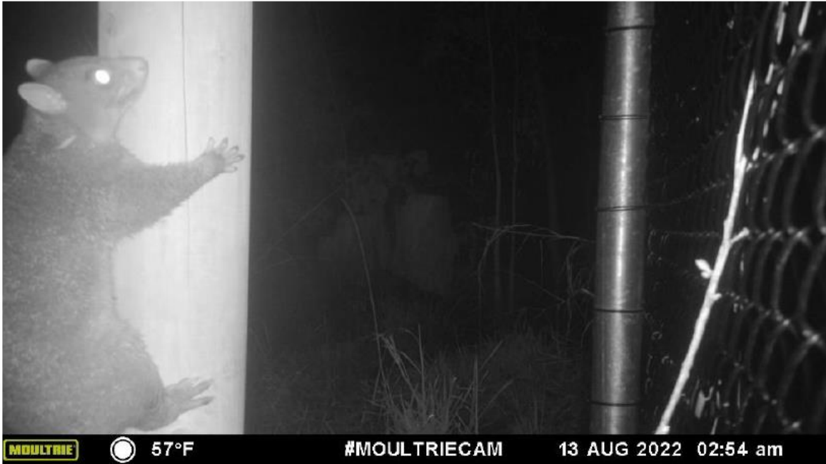
Figure 3: Infrared camera capture of a Short-Eared Brushtail Possum using a fauna escape pole
