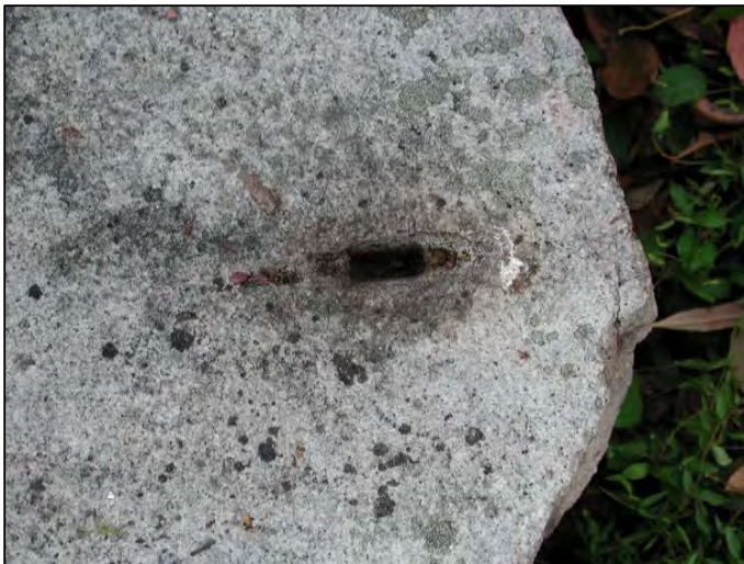
Figure 8. Sandstone block with rectangular hole possibly the result of attempts to split the block with gads. This hole is cratered at its upper edges, typical of the damage done when using gads.
