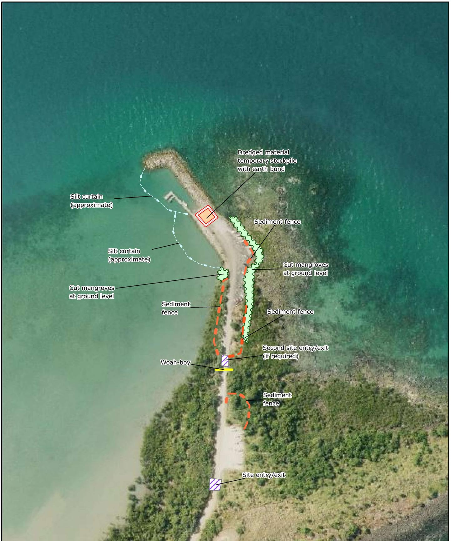
**Figure 3:** Temporary erosion and sediment control measures
