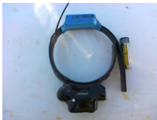
Figure 4. Koala monitoring collar with AAA battery for scale.
