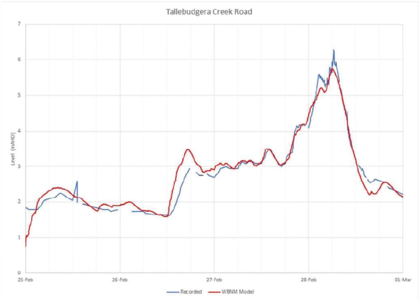
32 These results are consistently good. The modelled results closely mimic the recorded levels, providing a high level of confidence that the WBNM hydrologic model is accurately transforming actual rainfalls into measured flow rates.
