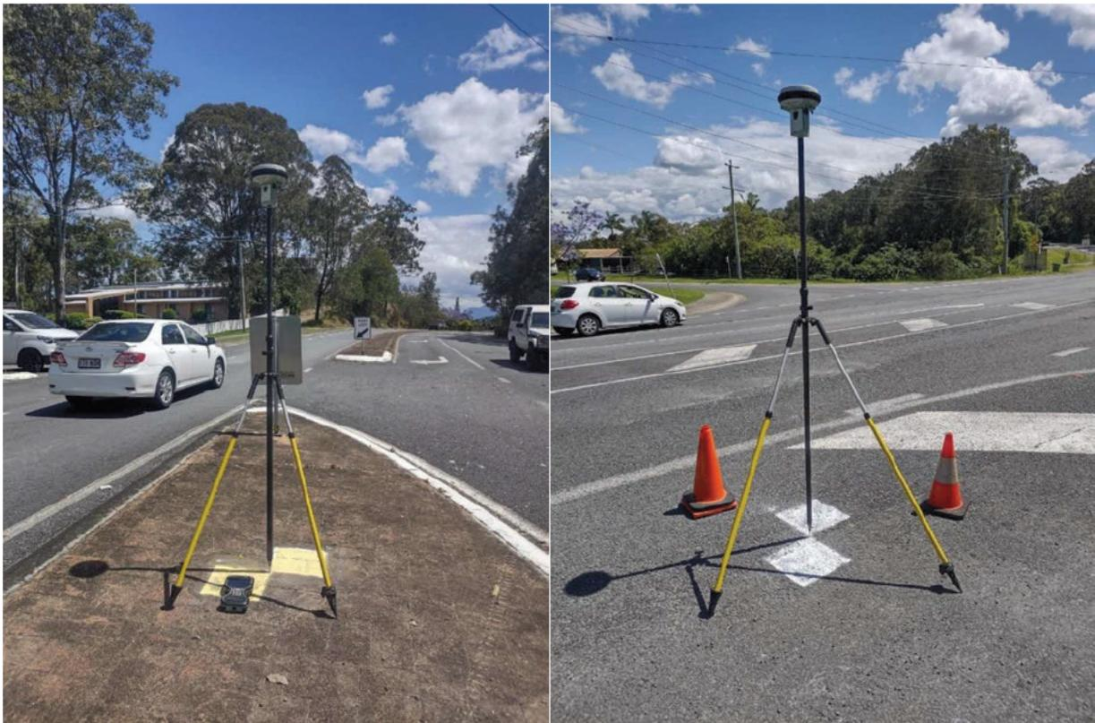
Picture 1 – Examples of Ground Control GCP01 & GCP02 as placed and observed
