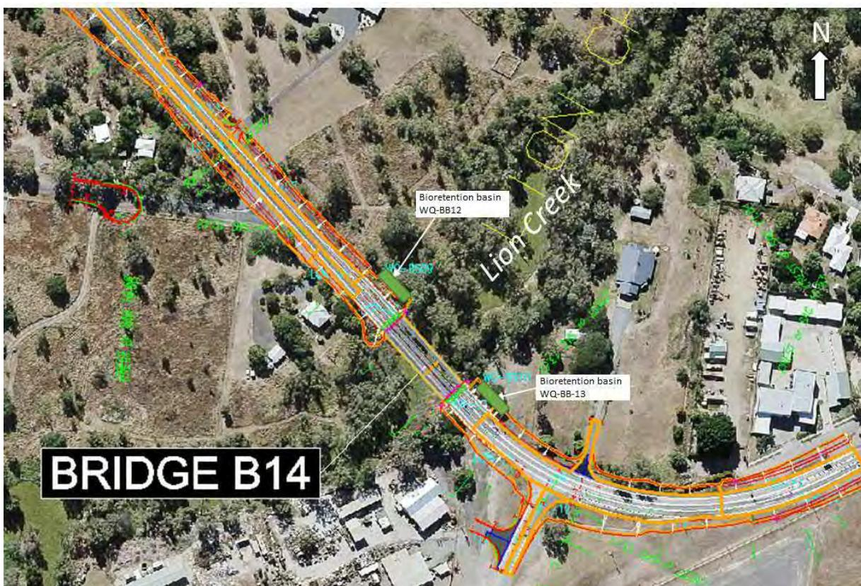
**Figure 10 Proposed bioretention swales at Lion Creek in RCR Zone**
