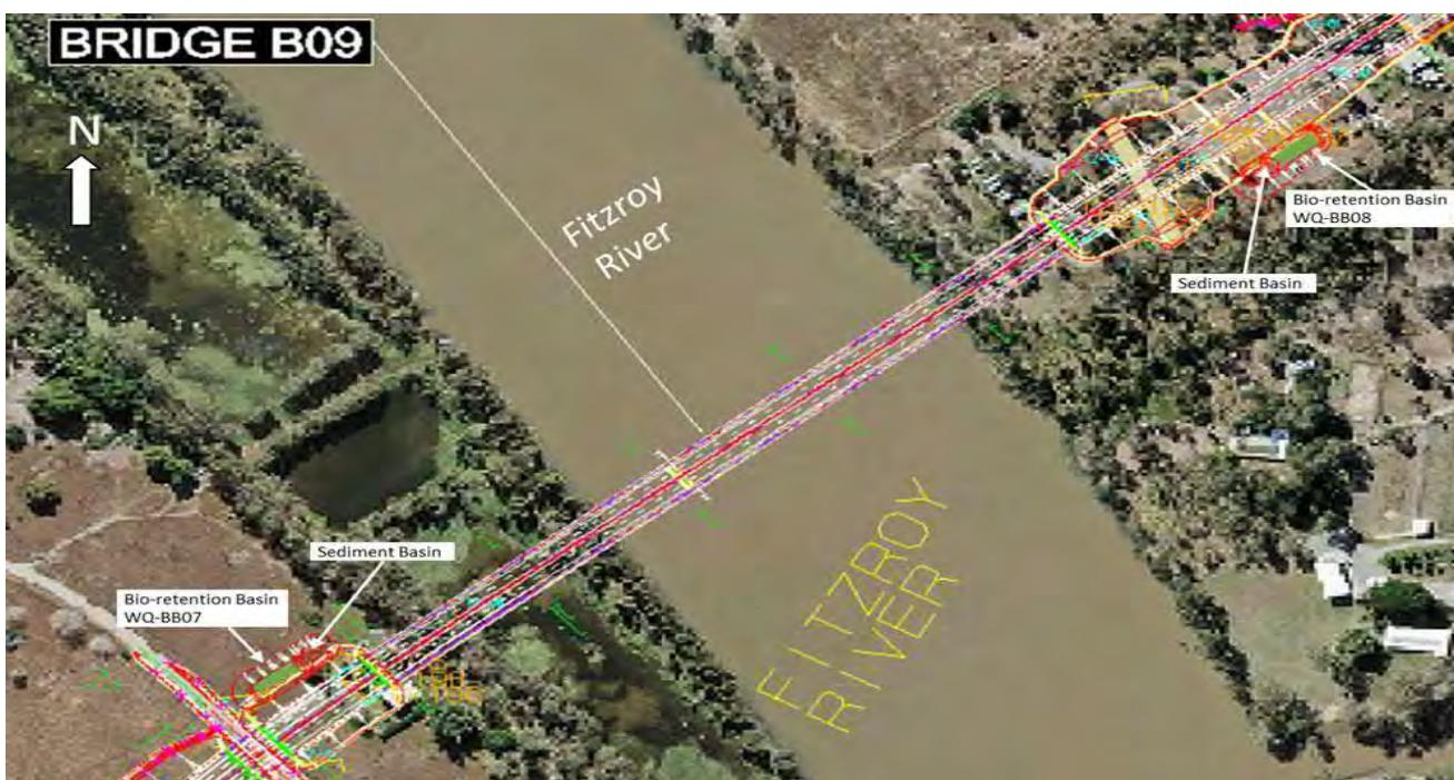
**Figure 2: Bioretention basins location at the Fitzroy River**
