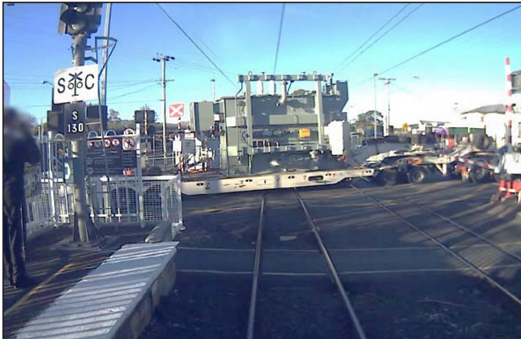
Figure 8: Heavy vehicle grounded on the level crossing, the CSA to the left on the radio
