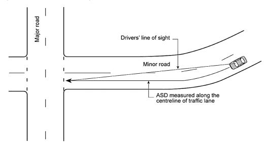
Figure 4.10(b) – Plan view of Safe Intersection Sight Distance (Source: Austroads 2021a)
