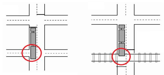
*Figure 4.9(a) – Examples of inadequate approach and departure stacking distances (Source: TMR 2013)*
