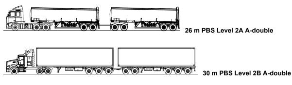
PBS-approved Level 2B A-doubles up to 30 metres overall length have on-road performance that is equivalent or better than conventional 26 metre B-doubles, with the exception of their high-speed dynamic performance, and bridge loading impacts.
