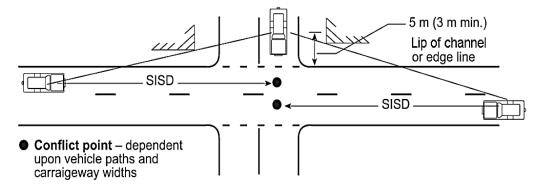
Prior Transport and Main Roads publications listed ASDs and SISDs, but not MGSDs, for B-doubles, and Type 1 and Type 2 road trains, for varying grades and travel speeds. Comparison of those values against the results of an Austroads heavy vehicle braking study (Austroads 2009b) shows that they are applicable to vehicles approved under the PBS scheme, and existing 'as-of-right' combinations.
