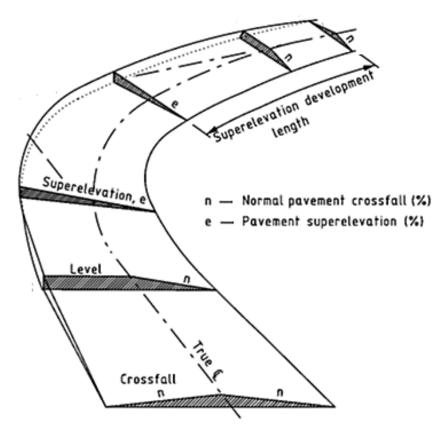
Figure 4.6 – Typical superelevation profile on two lane roads (Source: Austroads 2010)
