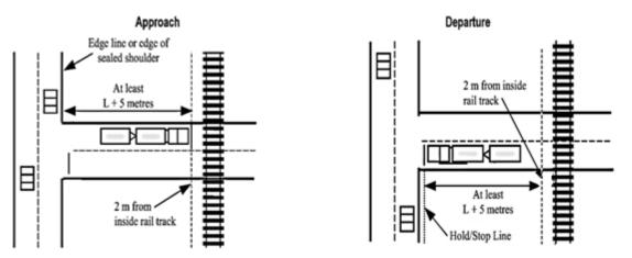
*Figure 4.9(c) – Minimum stacking distance requirement for intersections (Sources: NTC 2007 and AS 1742.7:2016)*
