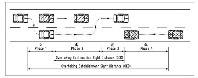
The establishment and continuation sight distances were studied by Transport and Main Roads (SMEC 2015), and the recommended minimum values are shown in Table 4.12(b) and Table 4.12(c) respectively.
