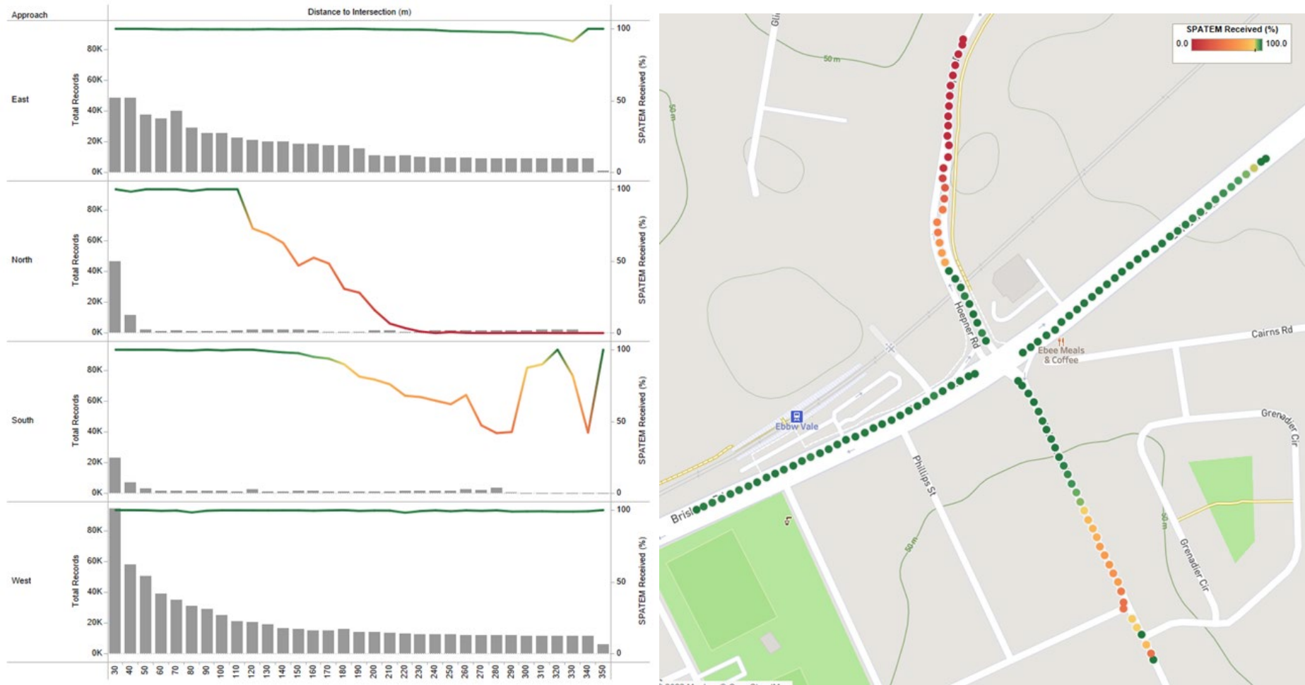
Figure 7.1(c) – Brisbane Rd / Hoepner Rd intersection - SPATEM range and associated coverage map
