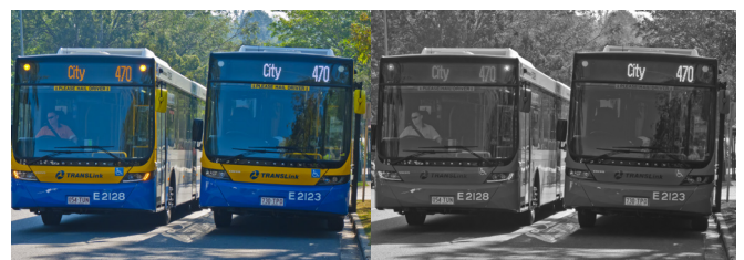
Figure 2.4 - Service-related signs must give the maximum contrast with their background for enhanced legibility. Left: Colour contrast between amber and white route signs. Right: Luminance contrast between amber and white route signs.
