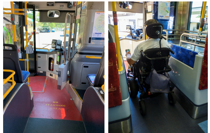
Figure 2.2 - The 'no standing area' illustrates the space which would benefit from being made as wide as possible to facilitate embarking and disembarking.
