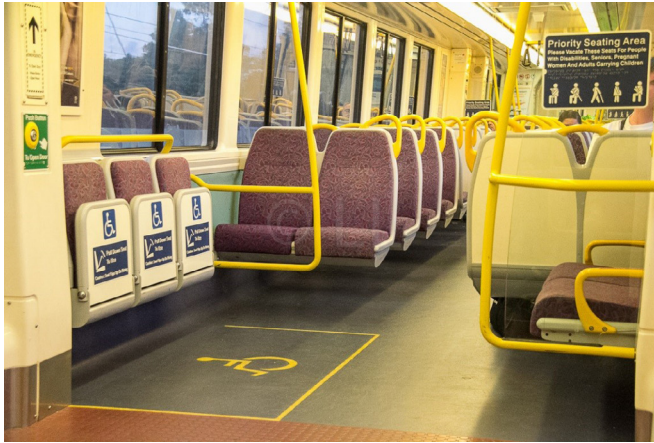
Figure 2.6 - A good example of a wide manoeuvring area, allowing passengers using a mobility aid enough access to manoeuvre even during peak periods. N.B. The international symbol of access on the floor would benefit from being the standard white on blue design as per the International Symbol of Access; to ensure this space can be universally and internationally recognised.
