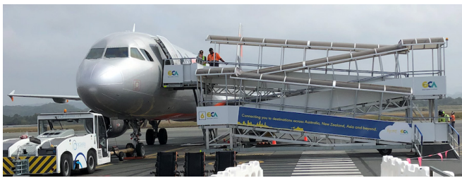
Figure 2.11 - 'Mega ramp' an alternative solution for airports without an airbridge. Adequate space should be provided in the rest areas on each level.
