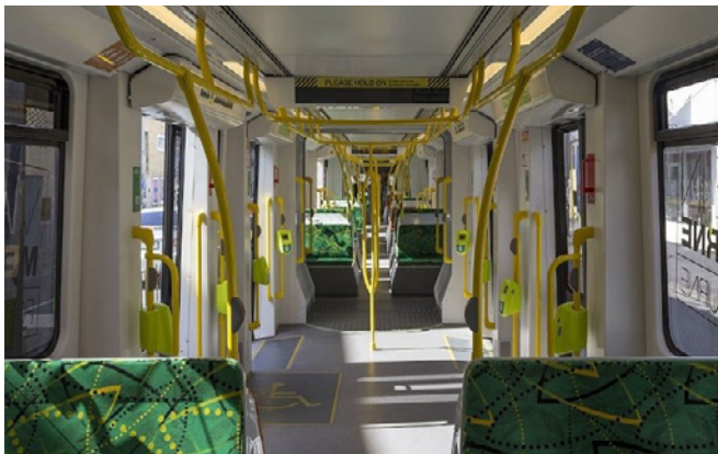
Figure 2.8 – An example of consistent handrail/grabrail colour and enough contrast throughout a light rail carriage.
