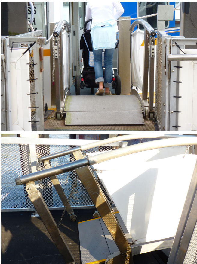
Figure 2.12 - The gangplank provides users with a gentle gradient when embarking and disembarking, due to its convex profile and better integration with the boarding surface.
