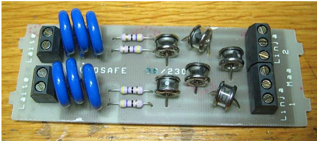
Figure 6.8.6(b) – Typical metal oxide varistors (blue) and gas discharge tubes (silver) for power circuit protection
