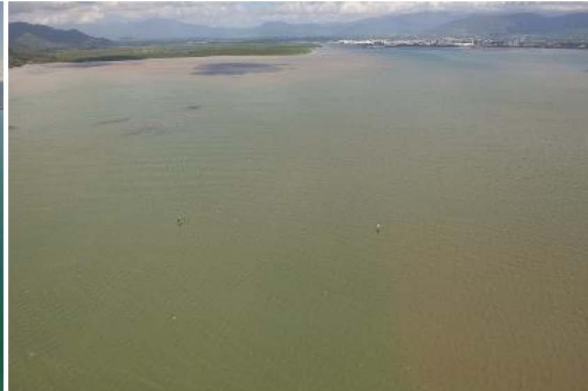
Photograph 2: Also taken during an ebbing tide, however on a day where there 15 knot south-easterly winds were present. The photograph illustrates the naturally high turbidity (40 NTU at beacon 10 at the time of the photograph) resulting from wave induced sediment resuspension. The photograph also illustrates the, by comparison, clean ebb tide waters flowing out of the main channel.
