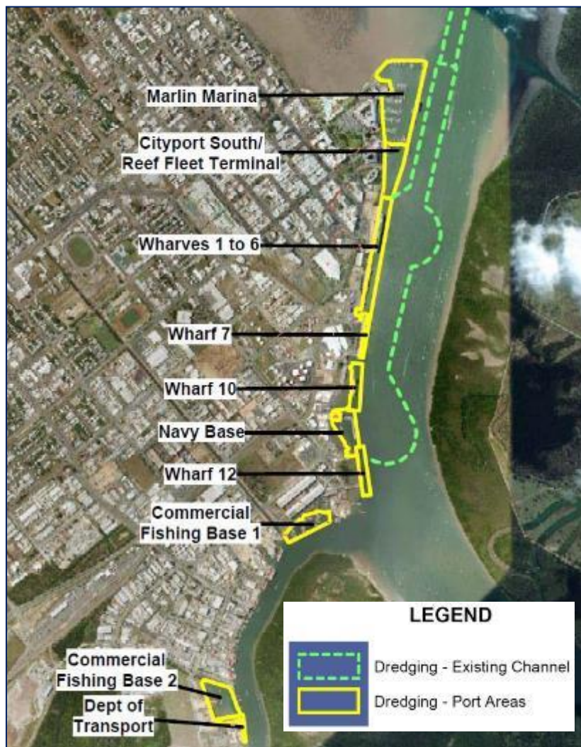
Figure 26: Extent of Maintenance Dredging Areas within the Port of Cairns (WorleyParsons, 2010b)
