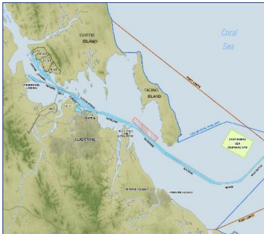
Figure 20: Extent of Maintenance Dredging Areas within the Port of Gladstone, blue area represents the gazetted channel while the red hatched area represents area of maintained depth for anchorage. (GPC, 2014b)
