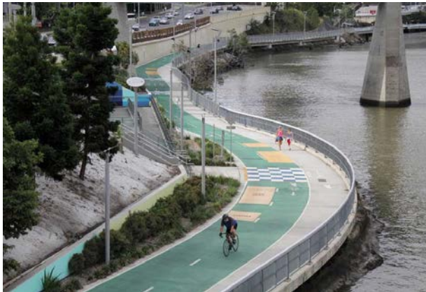
Figure 7-5: Example of a separated pedestrian and cycle path (Bicentennial Bikeway, Brisbane)
